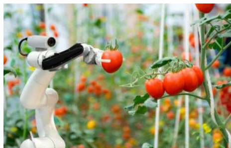
Figure 2: Robot harvesting tomatoes (Arreola et al, 2019)
